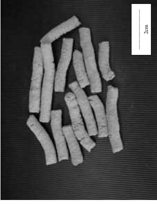
Fig. Micro-habitat pellets made from dredged sediments treated with AGOCLEAN-P (1.5%)
