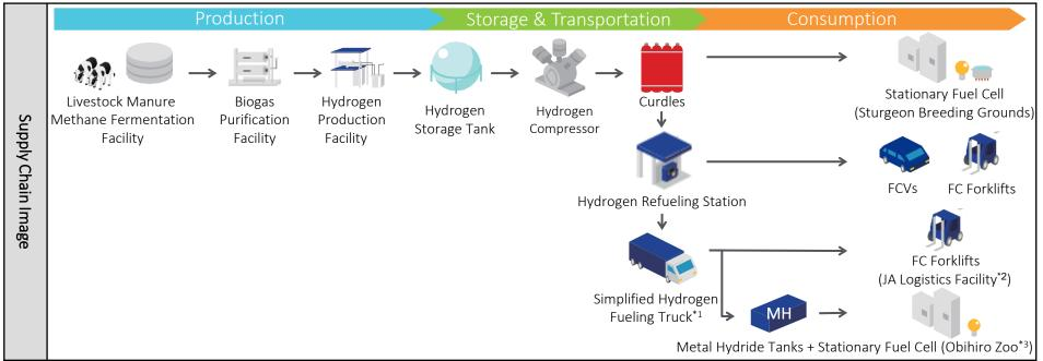
\*1 Use of simplified hydrogen fueling truck began in FY2021 \*2 Supplying by simplified hydrogen fueling truck to FC forklifts at a JA logistics facility has been conducted multiple times for a limited time period since FY2020. \*3 The metal hydride tanks with pure hydrogen fuel cells were installed at Obihiro Zoo in FY2020. Supplying for dairy facilities and sightseeing complex facility "Tokachimura" have ended as of FY2019. (Source: AIR WATER Inc. project documents)
