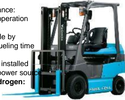
2.5 t Fuel Cell Forklift
