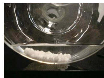
Fig.2.2 Photograph of NaOH/EG and balls in ball mill reactor
