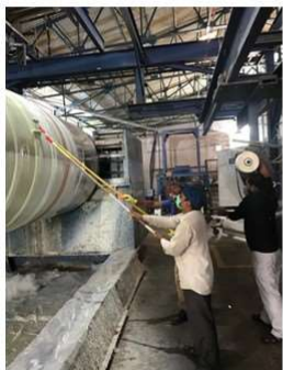
( A ) THE FRP UG TANK PROCESS ( CHOP HOOP WINDING PROCESS ).
