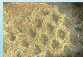
Clogging of filter media of contact aeration chamber (Example)
