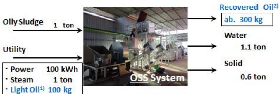
1) Using the light oil steam is produced by boiler. 2) The quality of recovered oil is dependent on kind of oily sludge.
