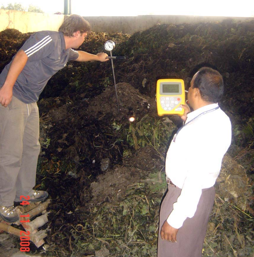
Regular Oxygen Monitoring
