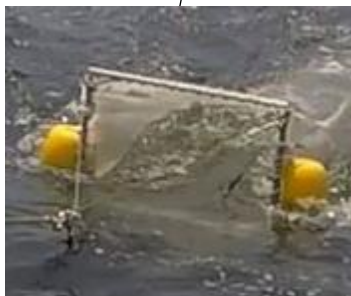
Immediately after tow starts (net immersion depth normal)
