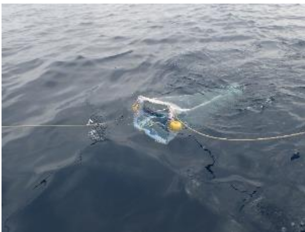
Fig.2-15. Adjustment of immersion depth of the Neuston net by attaching appropriate floats.
