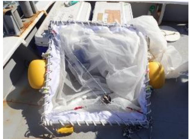
Neuston net with flow meter
