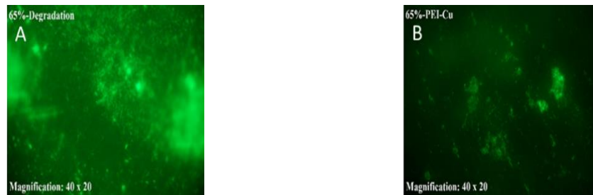
Fig. 3 Images observed using a fluorescence microscope after exposure to crossflow. (A) Degraded 65%-rejection membrane and (B) CuNP-coated membrane.
