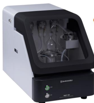
MAP-100 Microplastic Automatic Preparation Device
