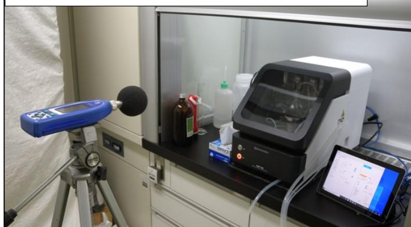
Measuring noise levels with an ordinary sound meter
