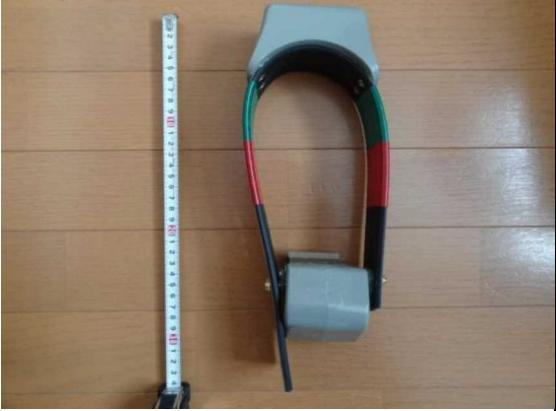
A photograph of the Vectronic GPSPLUSCollar2D GPS collar, which is a grey and black device with a red and green strap and a black antenna. It is shown from a side-on perspective next to a vertical tape measure. |
