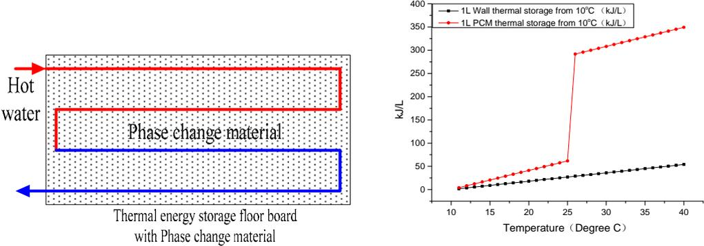
**Figure 2-24 Schematic diagram of thermal energy storage system with PCM**
