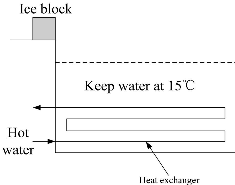
**Figure 2-26 Schematic diagram of ice block melting system**
