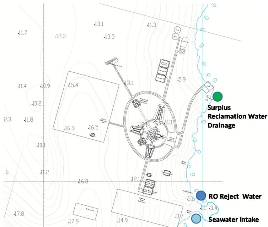
Figure 2-14 Intake and drainage locations
