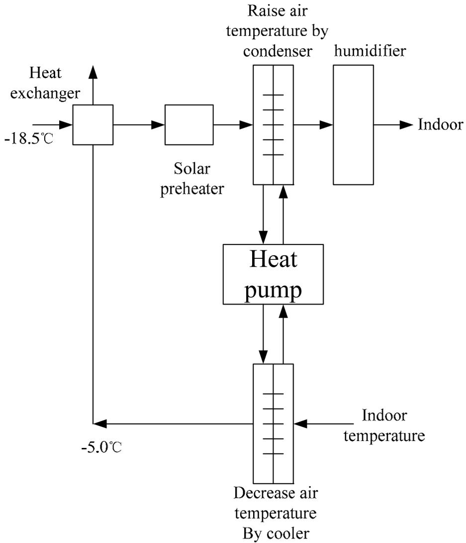
**Figure 2-25 Schematic diagram of fresh air preheating system**
