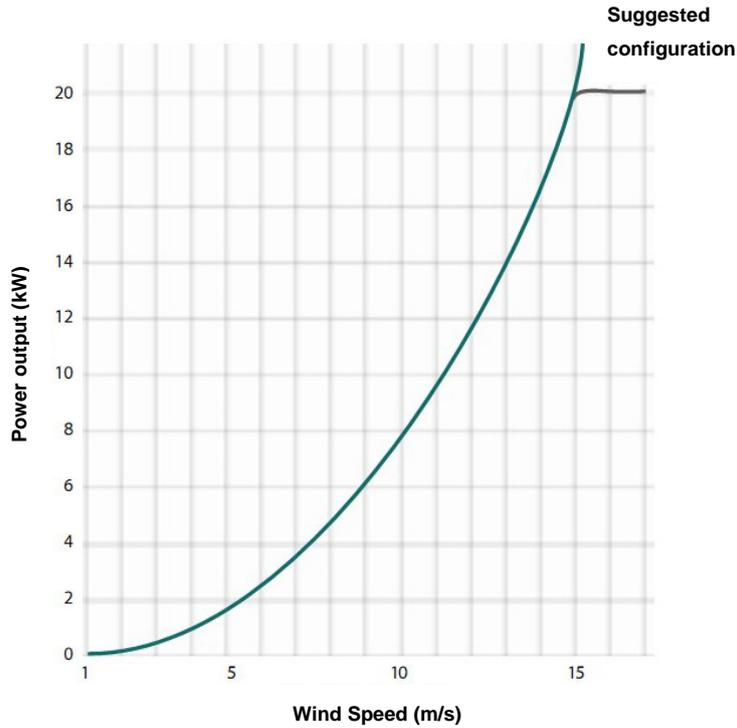
**Figure 2-21 Diagram of output power curve of UGE-9M**
