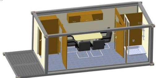
Figure 4 - Middle section of the module. Right-side view From the entrance: a lobby, wardrobe, catering zone, mini-kitchen, toilet, shower, water treatment, heating and storage area.
