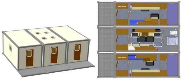
Figure 2.6 – General view (A) and layout (B) of the service & residential single-storey module
