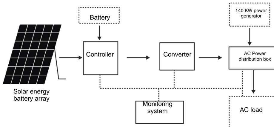
Fig. 24 Solar energy photovoltaic power generation system
