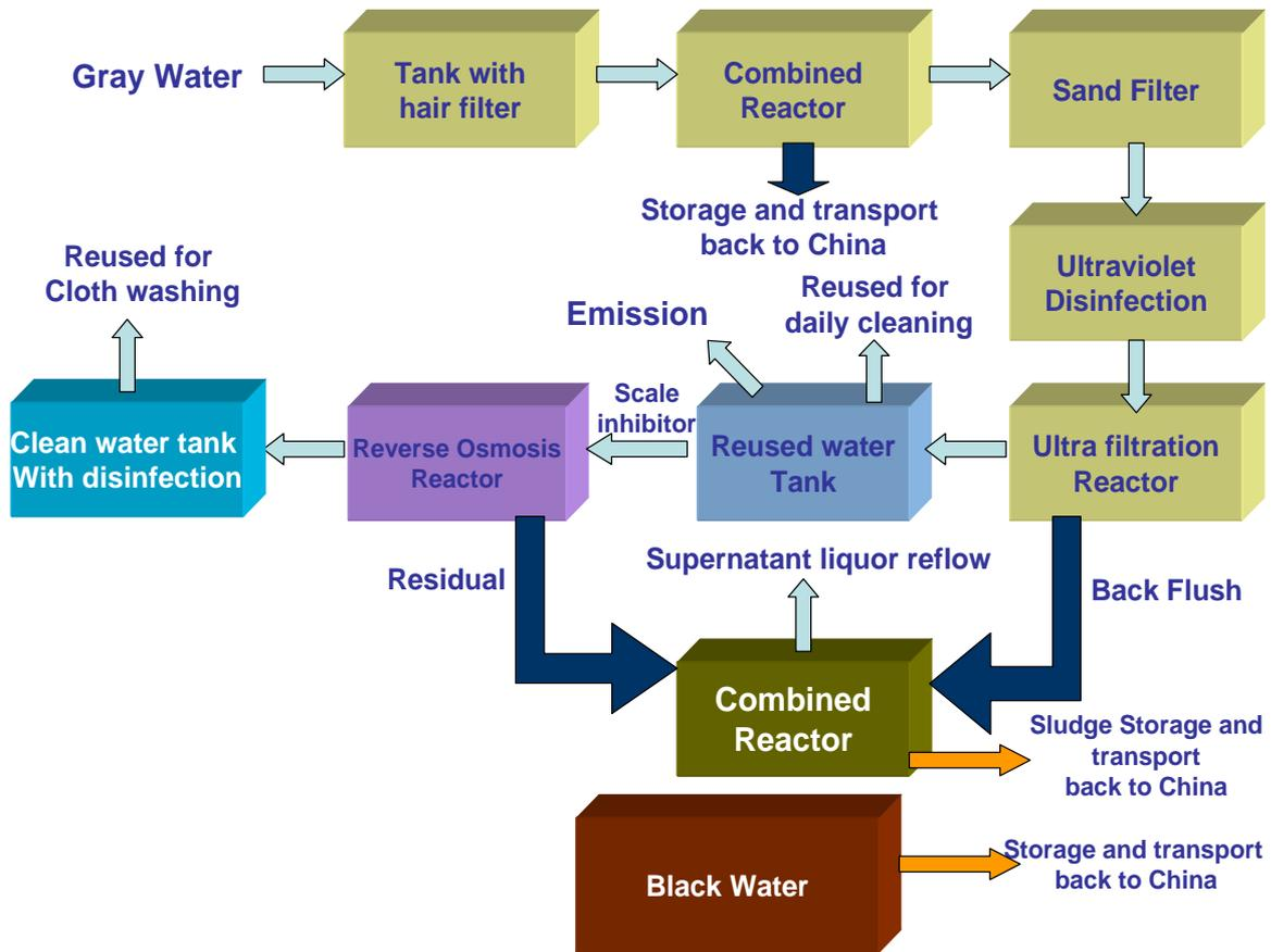
Fig. 23 Techniques for sewage treatment and recycling system
