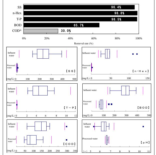
Note 1: The removal rate is determined by the equation shown below.
