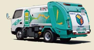
Low-pollution garbage collection trucks (Example) Generally, garbage loading and unloading is powered by the engine. This type of truck generates electricity required for loading and unloading while the truck is running. This reduces the consumption of light oil and CO<sub>2</sub> emissions.
