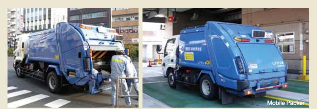
Safety, loading efficiency and operability are required for garbage collection trucks. Smaller trucks have openings set less than 800mm above the ground to realize outstanding workability and operability.
