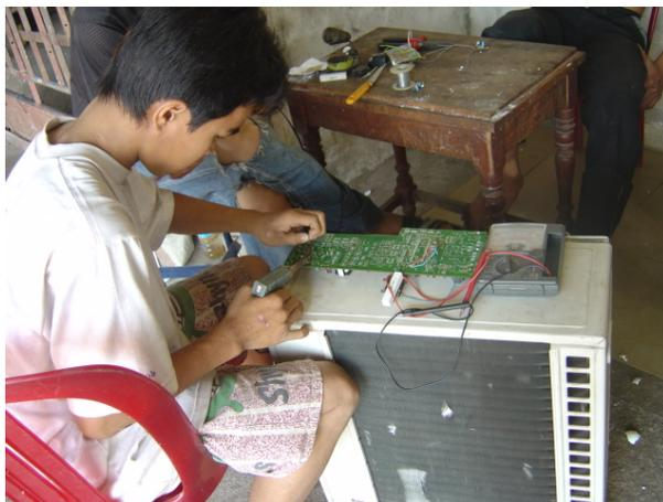
*Pic. 16: Simple methodology using for air-con repairing in Phnom Penh Municipality*
