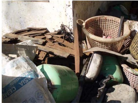
*Pic. 8: Improper keeping of gaseous block at scrap yard*
