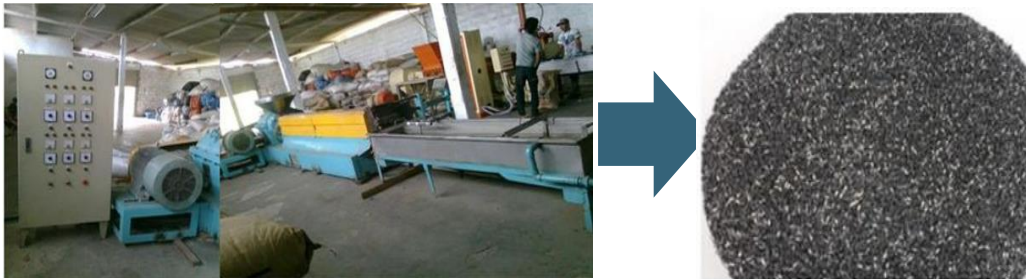
Pelleting process of plastic components in electronic waste
