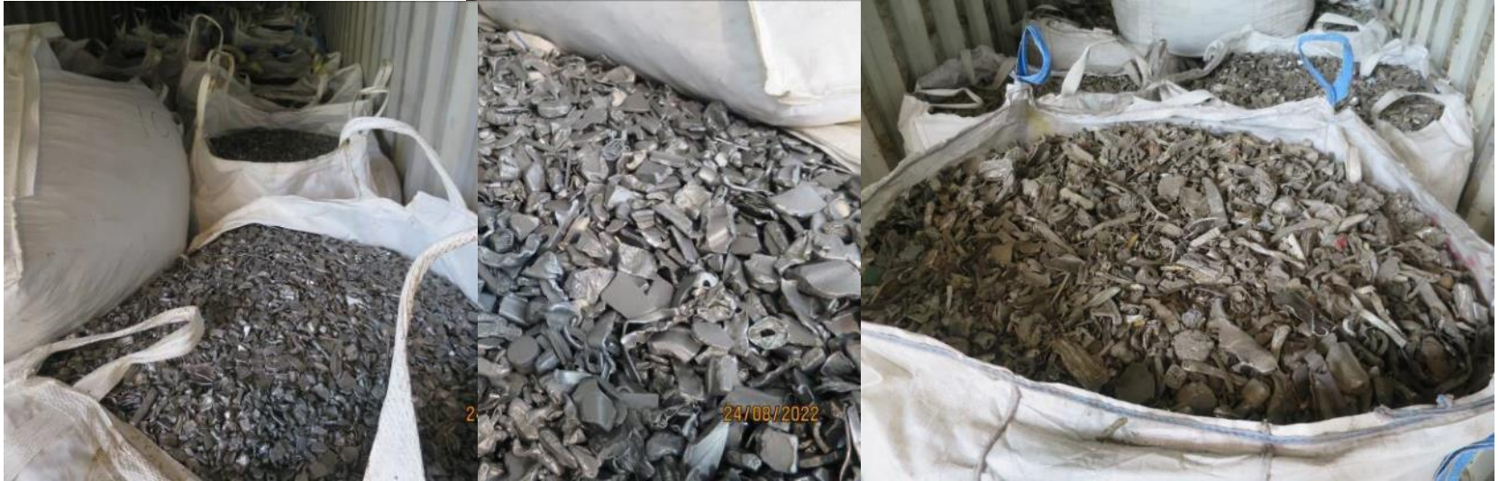
Uncontaminated Aluminium Scrap
