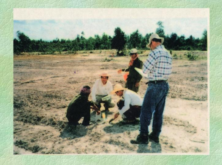
Checking the mercury concentration in soil after cleaning up and sampling the the ground water
