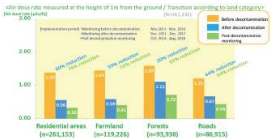
Air dose rates measured at the height of 1m above the ground / Transition according to land categories
