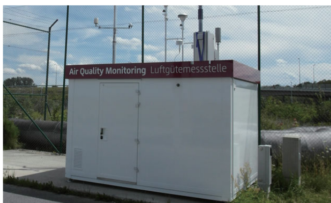
The air quality monitoring station in Berlin Brandenburg Airport This system includes our ambient monitoring analyzer, meteorograph and data logger.
