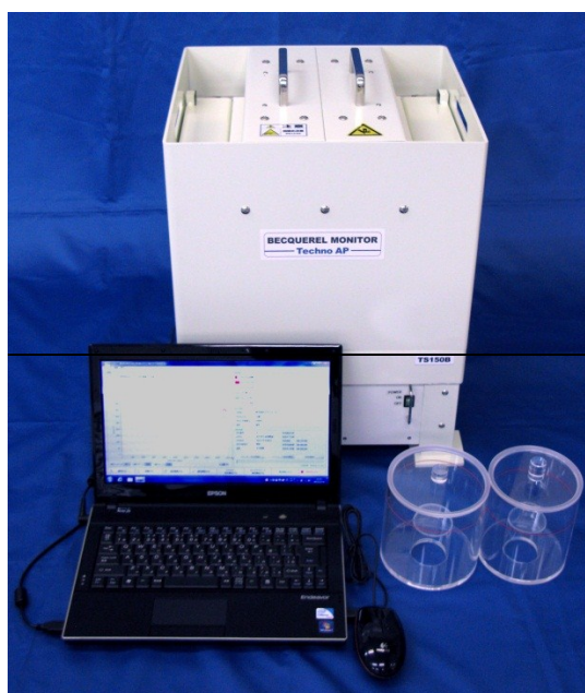
Figure 3-4-3 Example of a LaBr 3 (Ce) scintillation spectrometer
