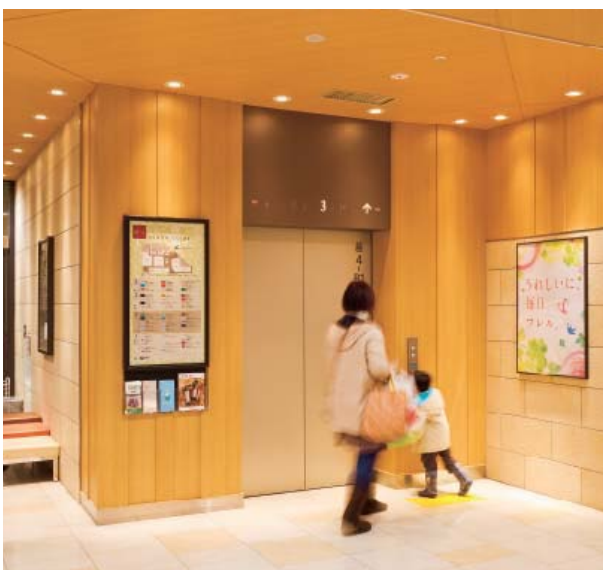
In the elevator hall, LED downlights project light towards the entrance and sign, drawing visitors' attention.
