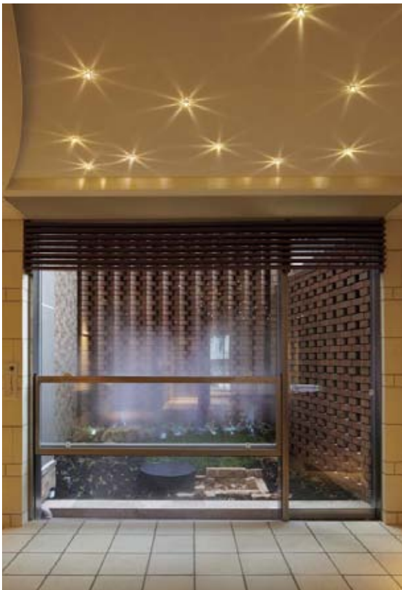
An evaporative cooler – an entirely natural cooling system – is installed in the courtyard facing the entrance hall. The lower window is designed to let fresh air into the hall – on the summer evenings, the Rokko Oroshi, a crisp wind that rolls in from nearby Mt Rokko cools the building.
