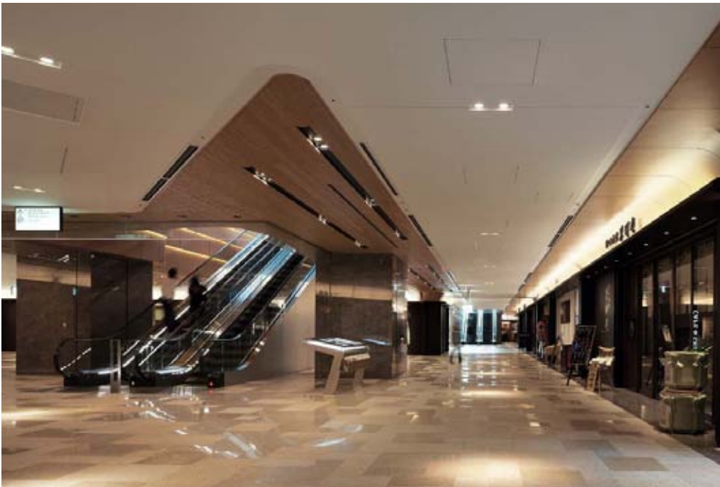
In the underground commercial area, continuous eave panels, where store signs are displayed and lit with indirect lighting, play an important role in unifying the passage design. The LED indirect lighting installed on top of the eaves has color temperature choice of yellow and white, which is adjusted by timer to create four types of lighting in the morning, afternoon, evening and night.
