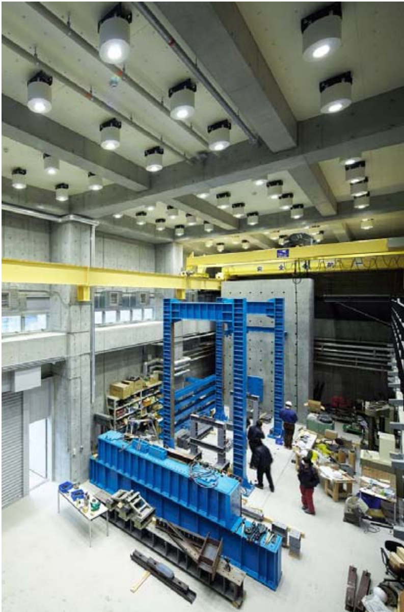
Structure laboratory. High-powered LED lights, with an output equivalent to the brightness of an HID lamp, are installed to provide even light distribution as well as reduce the maintenance costs normally involved in lighting a space with a high ceiling.
