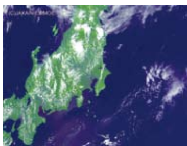
Figure 11. CAI Level 1B data collected on July 17, 2010 over the vicinity of mainland Japan. The image was produced by assigning colors (blue, red, and green) to the bands 1, 2, and 3.
