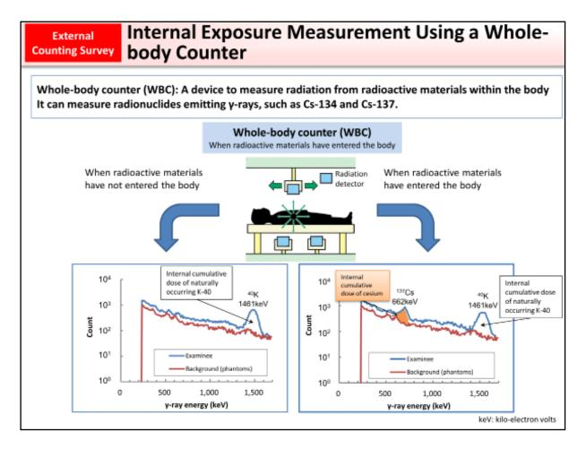
A whole-body counter is a device to measure  $\gamma$ -rays emitted from the body. As  $\gamma$ -ray energy differs by radionuclide, if a specific amount of energy, for example, 1,461 keV, which is the  $\gamma$ -ray energy of radioactive potassium (K-40), is counted, this can be interpreted as  $\gamma$ -rays emitted from K-40 in the body. The  $\gamma$ -ray energy of Cs-137 is 662 keV.
