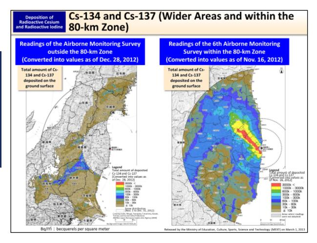
These maps show deposition of radioactive cesium on the soil surface in Fukushima and neighboring prefectures based on the readings of the airborne monitoring survey.
