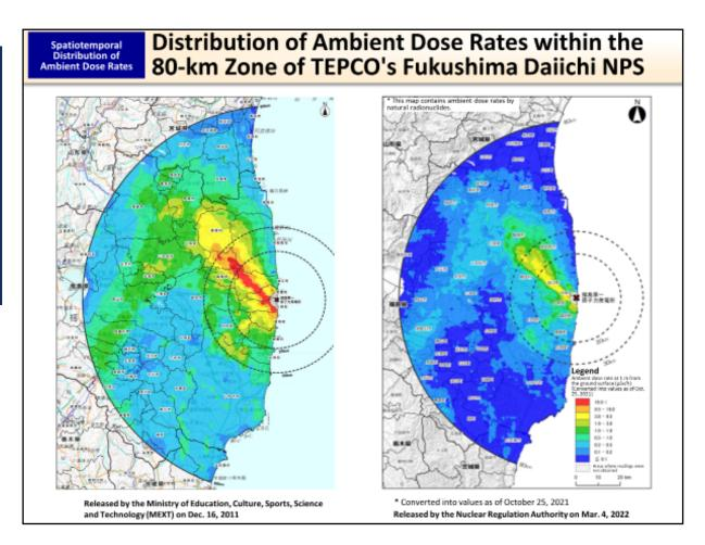
In order to ascertain the changes in the effect of radioactive materials, the airborne monitoring survey has been conducted continuously within the 80-km zone of Tokyo Electric Power Company (TEPCO)'s Fukushima Daiichi NPS, and the distribution of ambient dose rates and deposition of radioactive cesium have been surveyed. Additionally, the effect of radioactive materials outside the 80-km zone has also been ascertained through the airborne monitoring survey.
