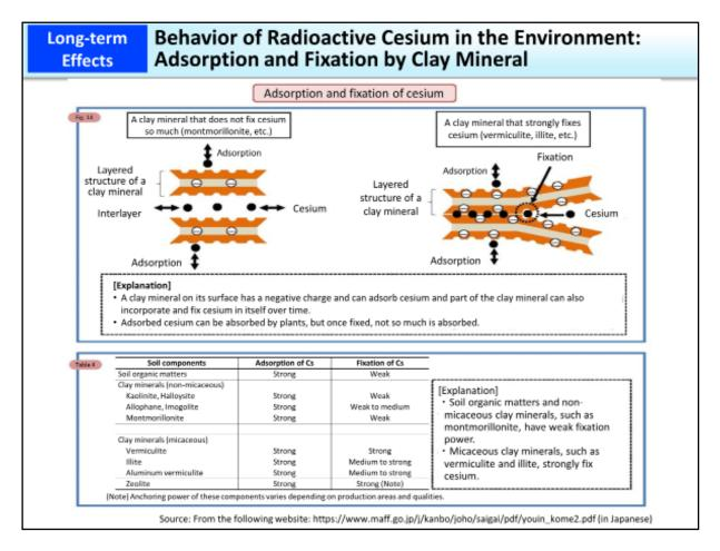
Cesium has a similar chemical property as potassium, etc. (having a positive charge) and can be easily adsorbed by clay minerals that have a negative charge superficially. Furthermore, some clay minerals have the ability to fix cesium that they have adsorbed, as time proceeds. It is known that cesium, once fixed, becomes hardly soluble in water.
