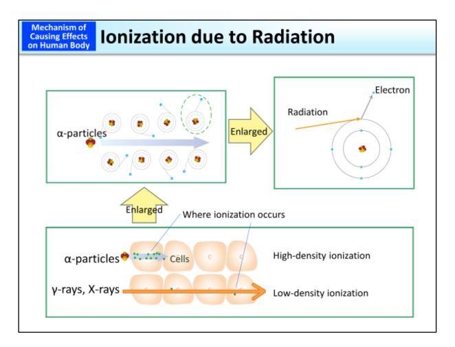
Radiation provides energy to substances along its pathway. Electrons of substances along the pathway are ejected with the given energy. This is ionization.
