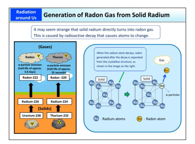
Radium, a radioactive material, is present in a crystal structure called body-centered cubic at room temperature and normal pressure, as shown in the right image.
