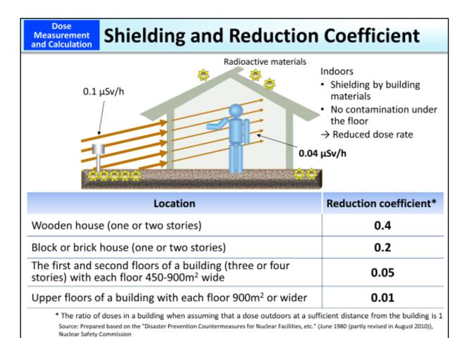
In the absence of an appropriate survey meter for measuring ambient dose rates (p.48 of Vol. 1, "Instruments for Measuring External Exposure"), calculations can be made based on the ambient dose rates that the government or local municipalities issued. For the amount of exposure outdoors, measurement results obtained near the relevant building are used. To calculate doses indoors, the indoor ambient dose rate is estimated by multiplying the value
