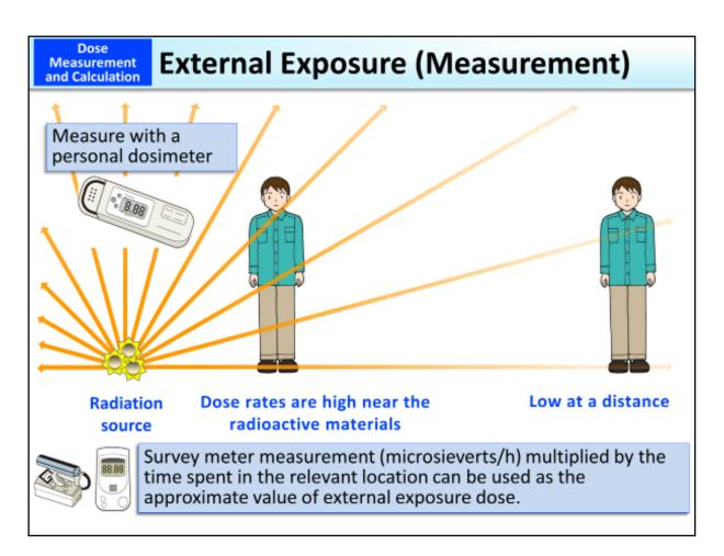
One of the means to measure doses due to external exposure is to wear a personal dosimeter on the body. Personal dosimeters can measure cumulative amounts of radiation exposure for a certain period of time, and provide dose rate readings.
