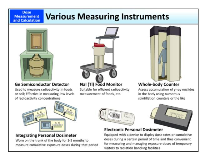
While radiation is not visible to the human eye, it is known to cause ionization and excitation (p.45 of Vol. 1, "Principles of Radiation Measurement"), and a variety of measuring instruments using these effects have been invented for different purposes and applications. The measuring instruments shown above all utilize the excitation effect.
