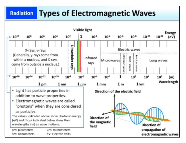
Electromagnetic waves are waves that propagate through space while an electric field and a magnetic field interact with each other. The shorter the wavelength is (the higher the frequency is), the higher the energy of an electromagnetic wave. The energy of radiation is expressed in electron volts (eV). 1 eV equals  $1.6 \times 10^{-19}$  Joule (J).
