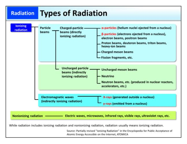
Radiation generally means ionizing radiation. Ionizing radiation, which has the ability to ionize atoms that make up a substance (separate the atoms into positively charged ions and negatively charged electrons), is categorized into particle beams and electromagnetic waves.
