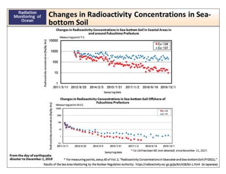
As a result of measuring dried sea-bottom soil samples collected in the coastal areas near Tokyo Electric Power Company (TEPCO)'s Fukushima Daiichi NPS, the concentrations of Cs-134 and Cs-137 were initially 1,000 Bq/kg but decreased in two years after the accident to 200 Bq/kg (down by 80%) and 500 Bq/kg (down by 50%), respectively. (Measuring Point T-1)
