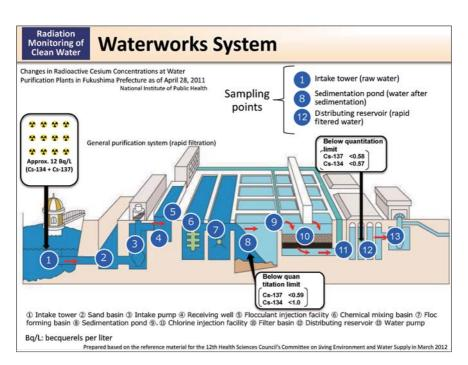
This figure shows the rapid filtration method, which is generally used in Japan. In this method, chemicals are injected into raw water taken from a river or dam to cause sedimentation of mud and small particles and make them into big chunks called "floc." Tap water is created by filtering the clear upper portion of such water.
