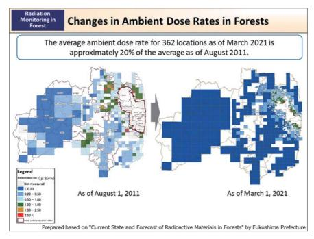
Fukushima Prefecture has been conducting monitoring of ambient dose rates in forests within the prefecture every year since FY2011. The monitoring targeted 362 locations in FY2011 but gradually expanded the coverage to target 1,300 locations in FY2020.
