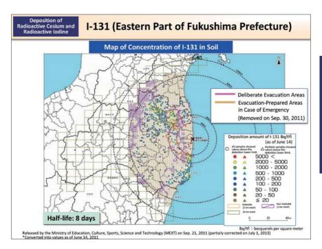
In the soil survey conducted by the national government in June 2011, three months after the accident, analysis of I-131 was conducted for soil samples collected within the 100-km zone of Tokyo Electric Power Company (TEPCO)'s Fukushima Daiichi NPS.
