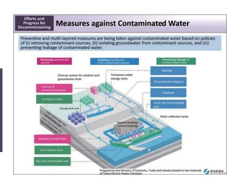
Water contaminated with radioactive materials has been treated based on the following three basic policies.
