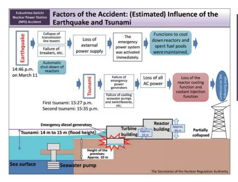
Immediately after the earthquake, at Units 1, 2 and 3 at Tokyo Electric Power Company (TEPCO)'s Fukushima Daiichi NPS, which were in operation, all reactors were shut down automatically.
