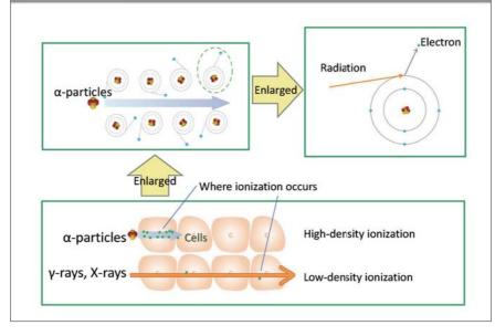
Radiation provides energy to substances along its pathway. Electrons of substances along the pathway are ejected with the given energy. This is ionization.
