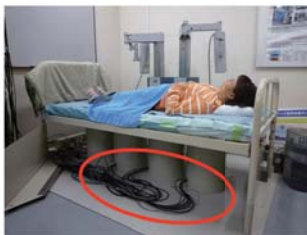
Scanning bed whole-body counter
