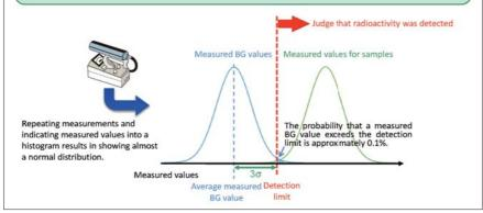
When measuring background radioactivity or dose rates using a survey meter or other equipment, even a minor change in measurement conditions can influence measurement results. Therefore, it is necessary to repeat measurements in order to obtain reliable measurement results.
