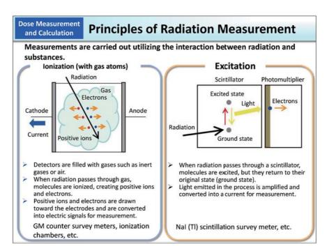
Radiation is known to interact with substances when passing through them. The amount of radiation can be measured utilizing the interaction between radiation and substances.
