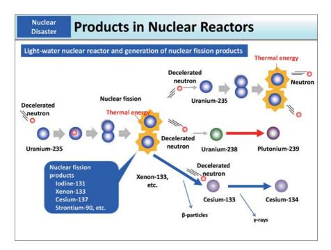
The light-water nuclear reactor is currently the most widely used type of reactor around the world (also used at Tokyo Electric Power Company (TEPCO)'s Fukushima Daiichi NPS). Bombarding enriched uranium fuel (Uranium-235: 3-5%; Uranium-238: 95-97%) with neutrons results in nuclear fission. Radioactive nuclear fission products such as lodine-131, Cesium-137, and Strontium-90 are created in this process. When Uranium-238 is bombarded with neutrons, Plutonium-239 is created.
