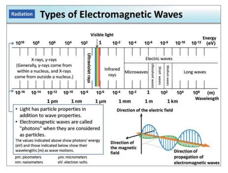
Electromagnetic waves are waves that propagate through space while an electric field and a magnetic field interact with each other. The shorter the wavelength is (the higher the frequency is), the higher the energy of an electromagnetic wave. The energy of radiation is expressed in electron volts (eV). 1 eV equals  $1.6 \times 10^{-19}$  Joule (J).
