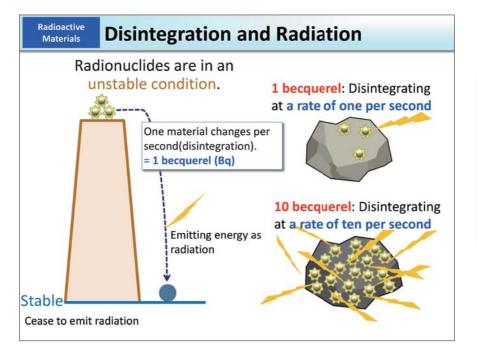
A nucleus of a radionuclide is energetically unstable. In order to become stable, it releases extra energy in the form of radiation.
