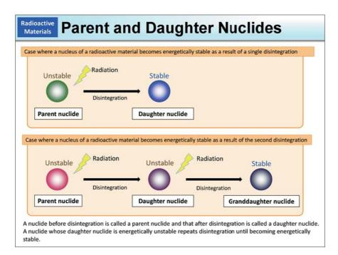
Types of atoms and nuclei classified depending on the number of protons and neutrons are called nuclides. For example, Carbon-12 and Carbon-14 are both carbons but are different nuclides. Carbon-14 is a radionuclide as it is energetically unstable.
