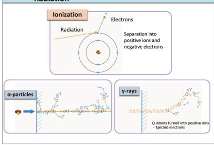
When radiation passes through a substance, its energy causes ejection of orbital electrons of the atoms that make up the substance, separating the atoms into positively charged atoms (or positive ion molecules) and free electrons. This is called ionization.
