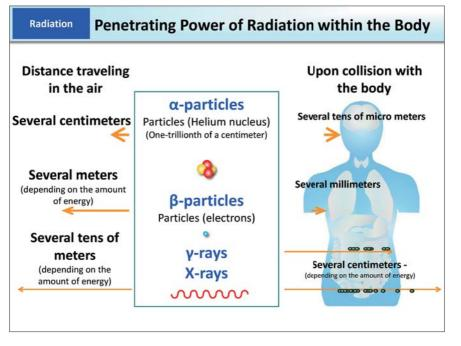
The easiness to penetrate through the air or the human body varies depending on the types of radiation. Therefore, the types of radiation ( $\alpha$ -particles,  $\beta$ -particles, or  $\gamma$ -rays) and radioactive materials (nuclides) that cause problems differ for external exposure and internal exposure.
